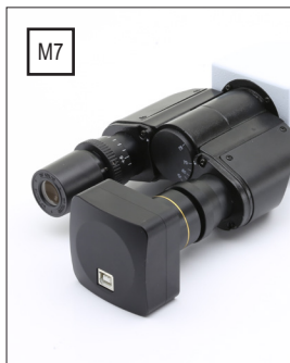
M7) Properly install the camera
