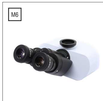
M6) Remove trinocular head's dust cover
