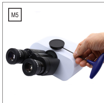
M5) Loose the clamping screw
