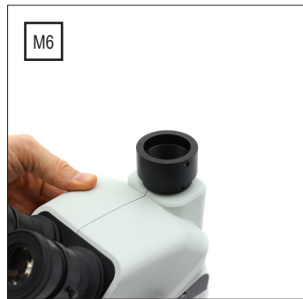
M6) Remove trinocular head's dust cover
