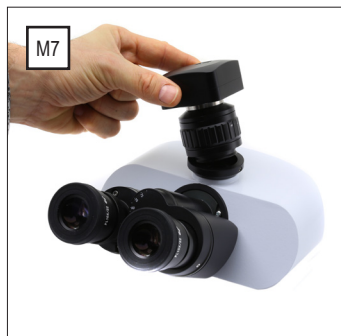
M7 / M8) Install the previously assembled C-mount + camera on the trinocular head
